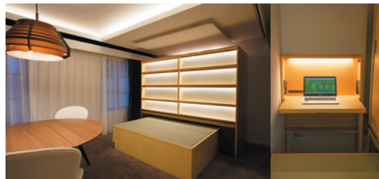
Figure 50: Robot furniture with storage function that separates the tatami-floored bedroom and the slightly raised telework space
