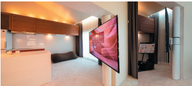
Figure 54: Automatically controlled movable TV stand that allows a single large TV to be used for various areas
