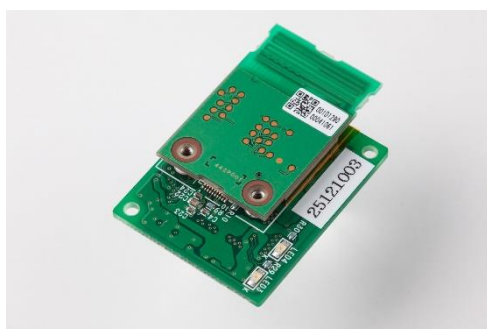
Figure 1-3 An example of wireless module that is joined to MPU module
