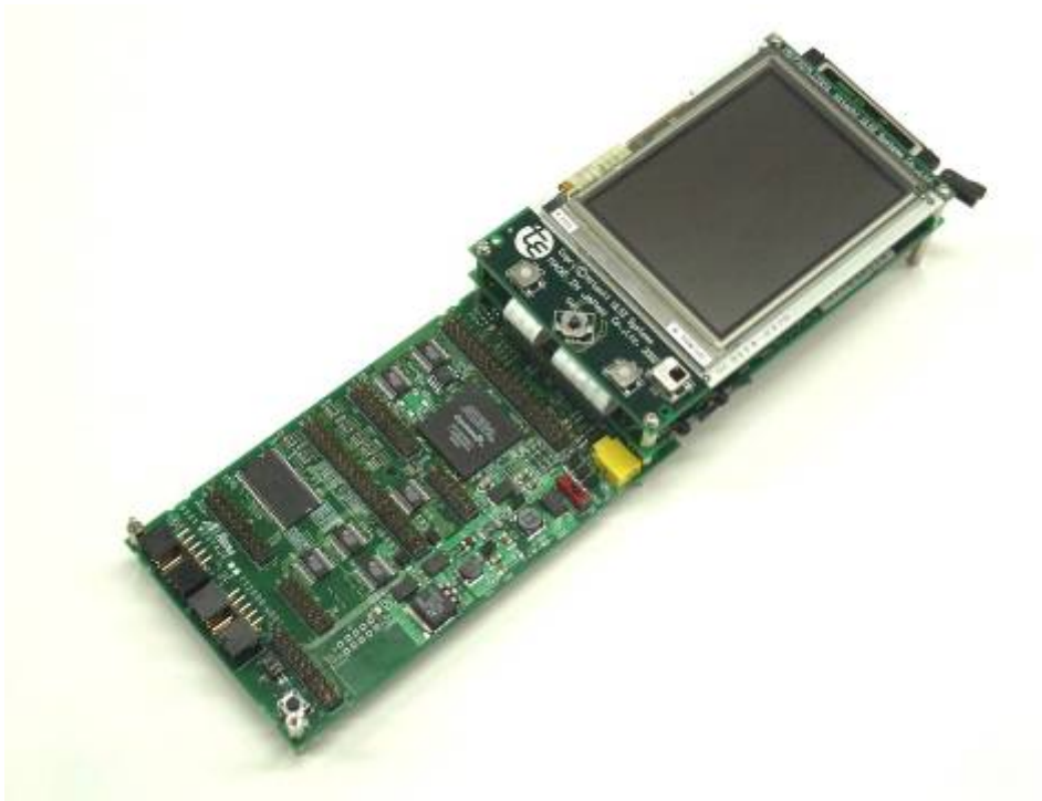
Figure 2.4.4: Structure of Expansion FPGA board manufactured by ALTIMA
