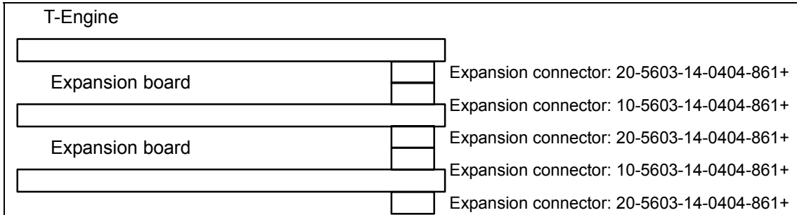
Figure 7.6.1: Expansion board stacking structure
