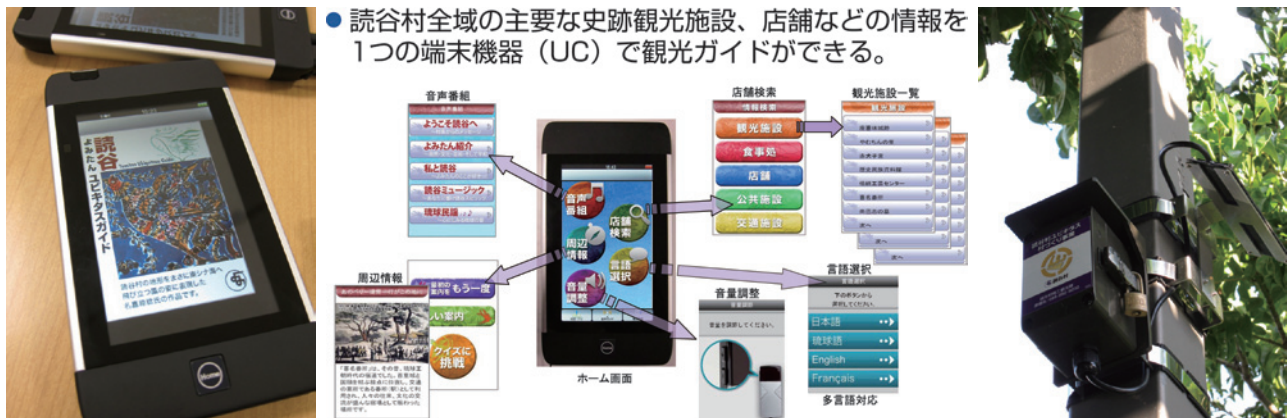
Figure 2.14 (Left) Terminal for Yomitan Village Ubiquitous Guide System (middle) Outline of the Service of Yomitan Village Ubiquitous Guide System (right) Installed "ucode" Wireless Marker
