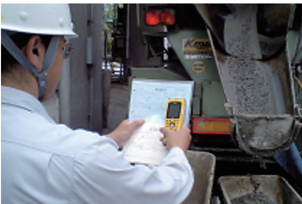
Figure 2.21 Fresh Concrete Quality Assurance Information System in Use
