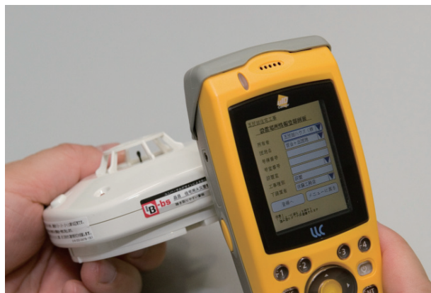
Traceability Management System of the Housing Components
